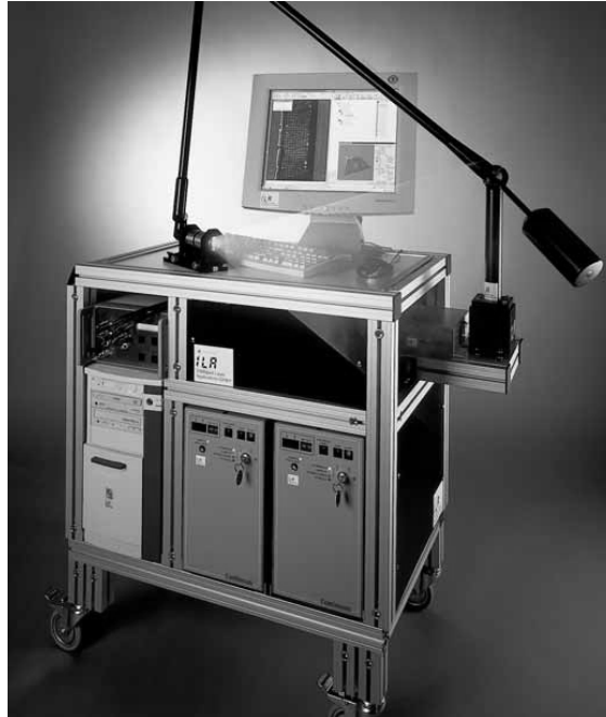
Fig. 3. Mobile 2D-PIV system from ILA [11].
