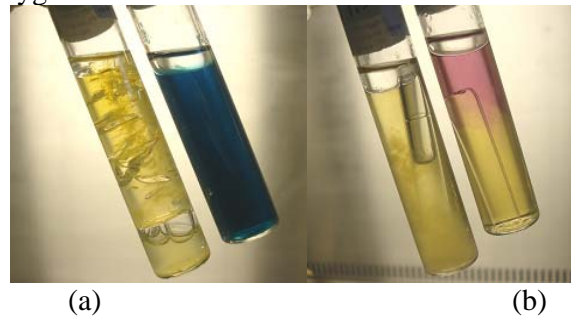
Fig. 2. Positive and negative tubes for acidogens (a) and methanogens (b) analysis
