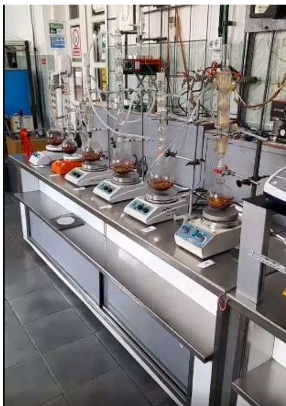
Fig. 2. Perfect mixing reactors used for impregnating shredded vine residues with H_3PO_4 solutions.
