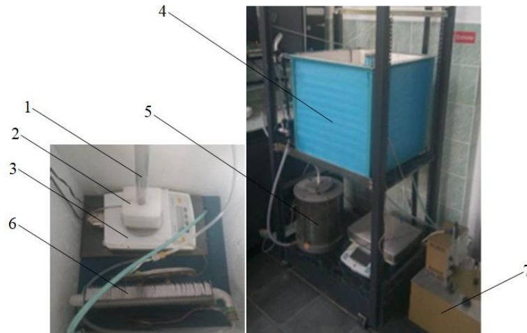
Fig. 4. Adsorption setup: (1) glass adsorption column; (2) holder; (3) digital balance; (4) insulating enclosure; (5) silica gel column; (6) finned heater; (7) water bath.
