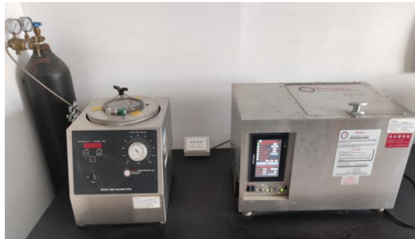
Fig. 2. PAV Pressure Aging Tester
