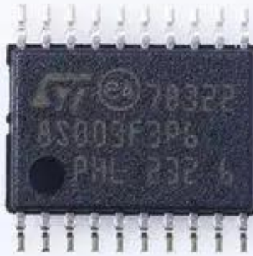
Fig. 2 The single-chip microcomputer (STM8S003F3P6TR model)
