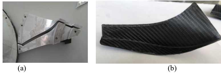
Fig. 2. (a) Two-component mould used to manufacture the (b) composite rotor blades
