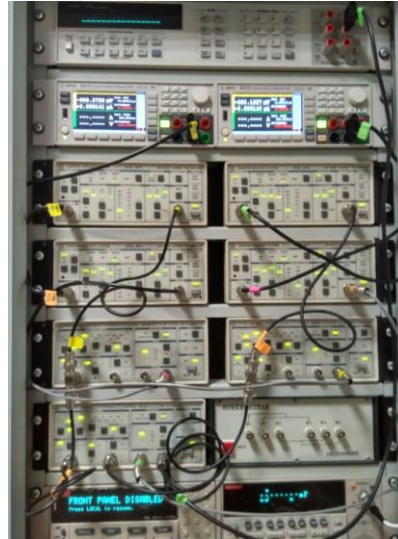
Fig.3 Hardware-in-the-Loop Simulation Platform of GGI
