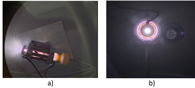
Fig.6 a) Top view of the HPT experimental prototype in CWM operation under 8 sccm of Argon and 200 W forwarded power; b) HPT plume plasma structure
