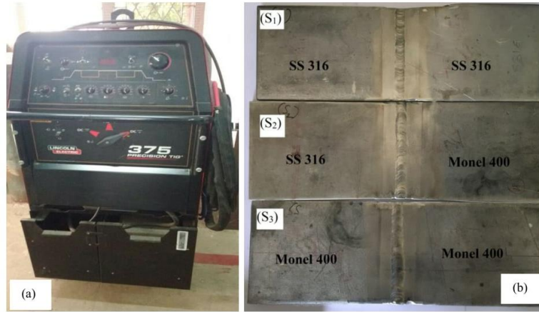
Fig. 2. (a) LINCON 375 manual welding machine, (b) Welded joints image (S 1 , S 2 and S 3 )
