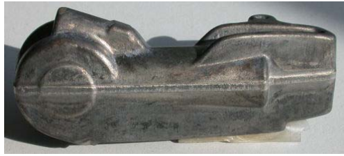
Fig. 1. Forged LEIBER bicycle part
