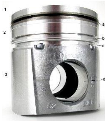
Fig.1. Components of a piston [1]: 1 - the piston head; 2 - port-segment region; 3 - the piston skirt.
