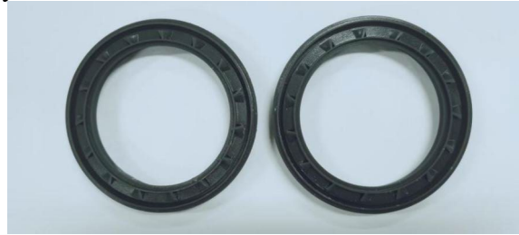
Fig.10 Physical model of the fan-shaped bearing dust cover
