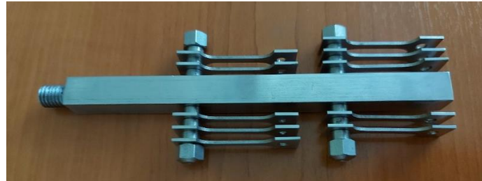
Fig. 3. The 316L sample holder for pre-exposure in the liquid lead environment.
