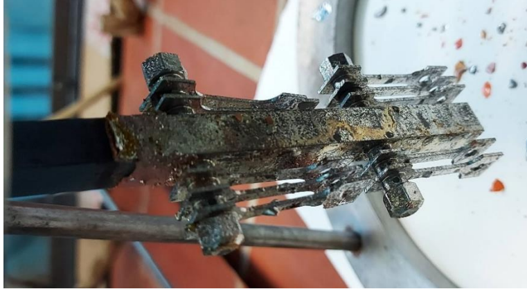
Fig. 4. Samples after exposure in liquid lead environment for 1000 hours
