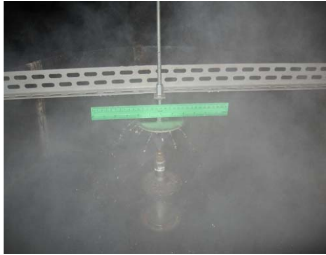
Fig. 10. Two phase jet at 40°C water temperature
