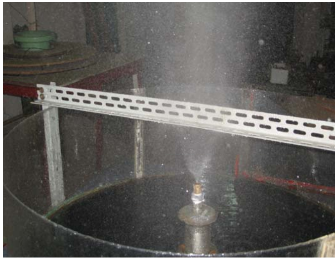
Fig. 9. Free two phase jet at 20 °C
