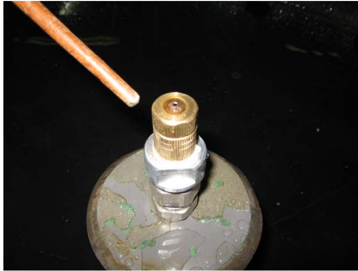
Fig. 7. View of the nozzle assembly water atomizer
