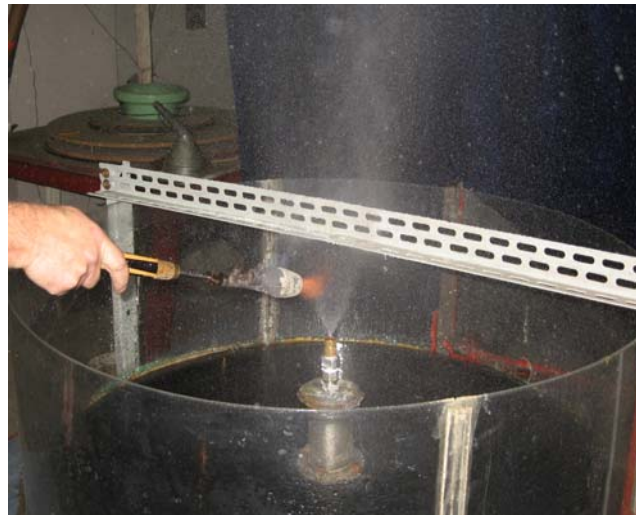
Fig. 11. Flame behaviour at the contact with the two-phase jet
