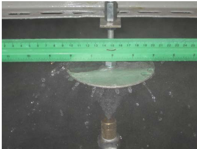
Fig. 8. Liquid jet development at 13°C water temperature
