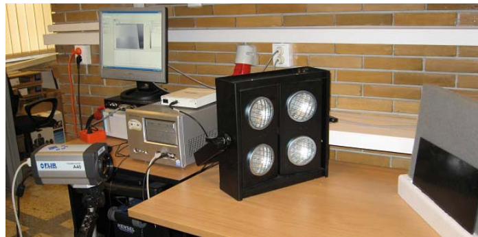
Fig. 4. The experimental setup for inspecting the CFRP specimens
