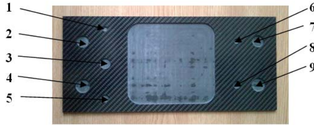
Fig. 2. CFRP plate with defects (thickness variation)
