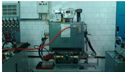
Fig. 11. Secondary sector of hydrostatic transmission – laboratory model.
