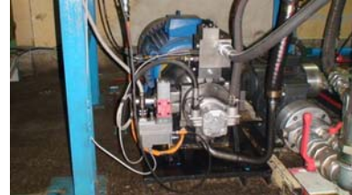
Fig. 10. Servo pump MOOG within the primary sector of hydrostatic transmission.
