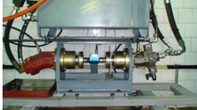
Fig. 9. Fixed pump for load simulation and Bosch adjustable motor within the secondary sector of hydrostatic transmission.
