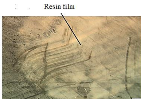
Fig. 2 Resin film over the analysis area of the dental milling cutter
