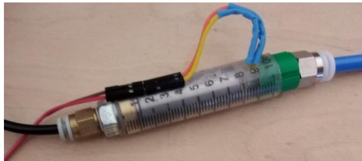
Fig.2. Pneumatic dispenser assembled in a syringe body.
