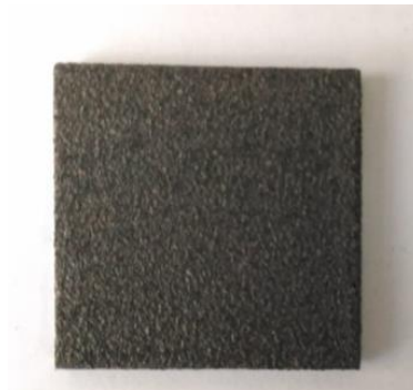
Fig. 8. Stainless steel sample, coated with \text{Co}_x\text{CrFeMoNi} high entropy alloy
