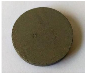
Fig. 5. Sample of \text{Co}_x\text{CrFeMoNi} high entropy alloy after compression testing
