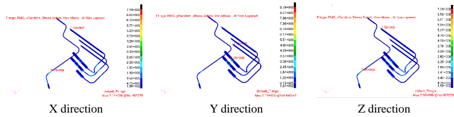
Fig. 8. Stress cloud diagrams of the heat pipe in three directions
