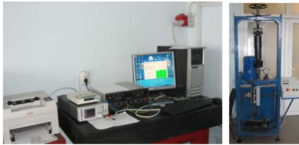
Fig. 6. Measurement equipment setup and test bench with hydraulic damper as load.
