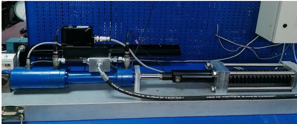
Fig. 9. Main view of the new dynamic test bench of the industrial servovalves developed in the FLUID POWER LABORATORY of the University POLITEHNICA of BUCHAREST [10]
