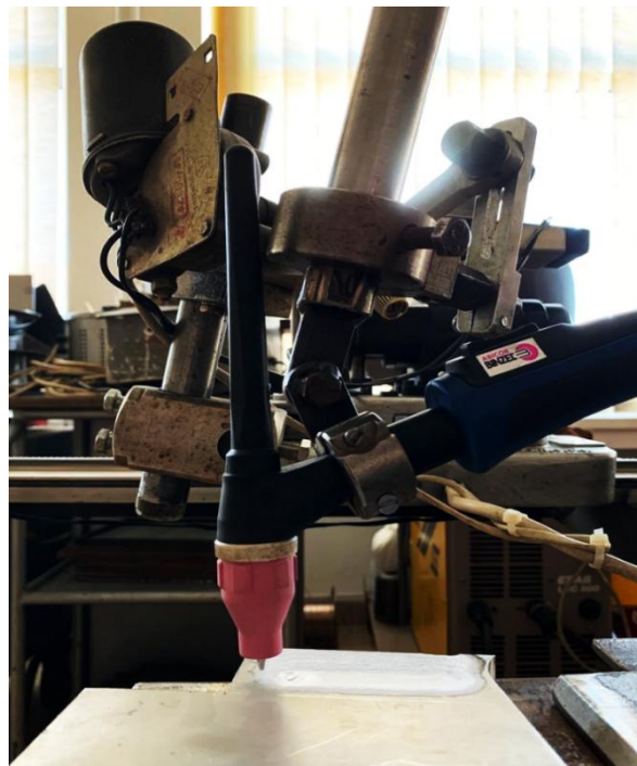
Fig. 1 Experimental stand used – TIG welding machine
