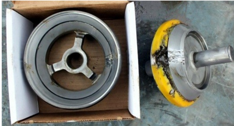
Fig. 4. Valve assembly affected by erosive wear (offshore platform)
