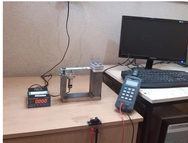
Fig. 1: Experimental setup for piezoresistivity measurement
