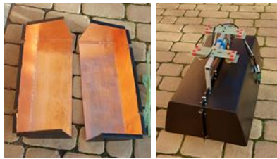
Fig. 5. Glass-textured protection covered inside with copper foil for GPR antenna
