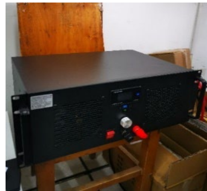
Fig. 4 Electronic load for test
