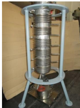
b) Melting vessel – electrical resistances distribution
