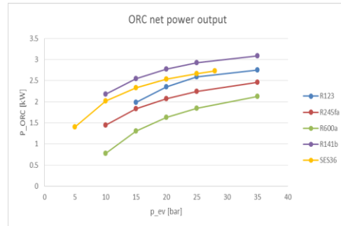
Fig. 5. Variation of net power output with evaporating pressure
