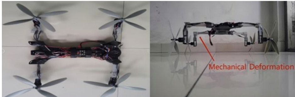
Fig. 1. The morphing quadrotor
