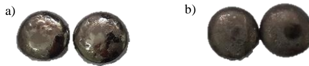
Fig. 4. Master alloys for Cu 45 Zr 45 Al 5 Ag 5 (a) and Cu 40 Zr 45 Al 5 Ag 10 (b)
