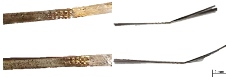
Fig. 2. Macro images of ultrasonic welded ribbons (upper view and cross-section view)
