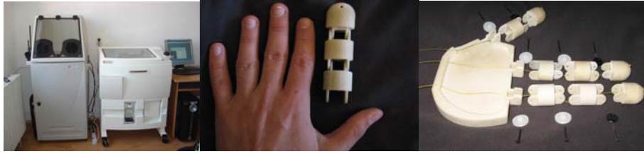
Fig. 3 – The 3D Zcorp printer used for fabricating the parts (left); finger and hand pictures before making the assembly (right)
