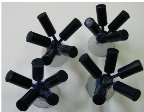
Fig. 1. Macroscopic aspect of experimental cobalt alloys samples after centrifugal casting
