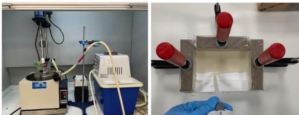
Fig. 1. The reactor used for prepolymer synthesis and the film casting process
