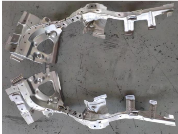
Fig. 11. This model of electric vehicle rear door reinforcement plate assembly product
