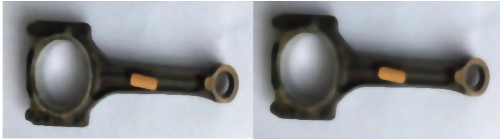
(c) Filter radius =5 (d) Filter radius =7 Fig.6 Connecting rod images processed with different filtering radii.
