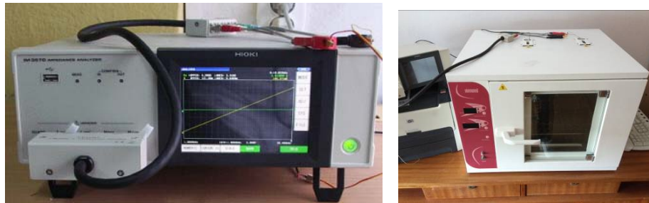
Fig.1. (left) Impedance analyzer used for the EMI technique type IM3570. (right) Heating chamber
