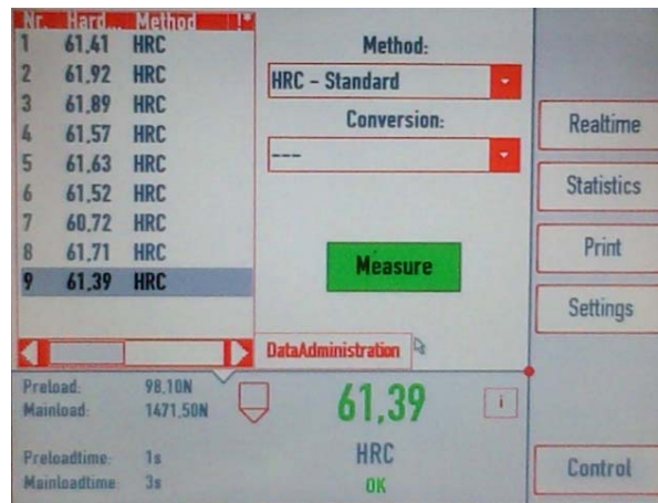
Fig. 3. Measured hardness on Rockwell type hardness tester CV-600A
