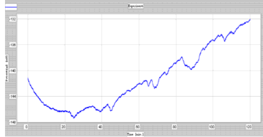
Fig. 2. The OCP versus time for Co-Cr-Mo alloy in Hank solution
