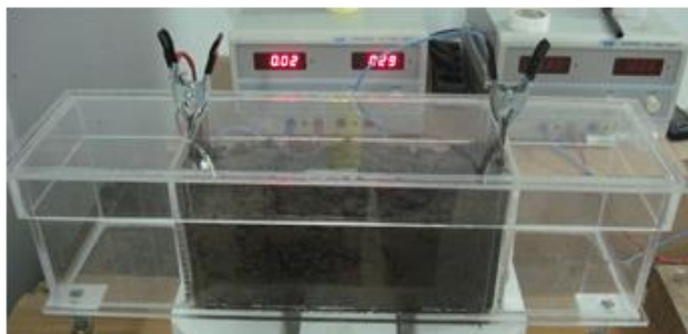
Fig. 1. The experimental setup used for the electrochemical treatment of the oil contaminated soil
