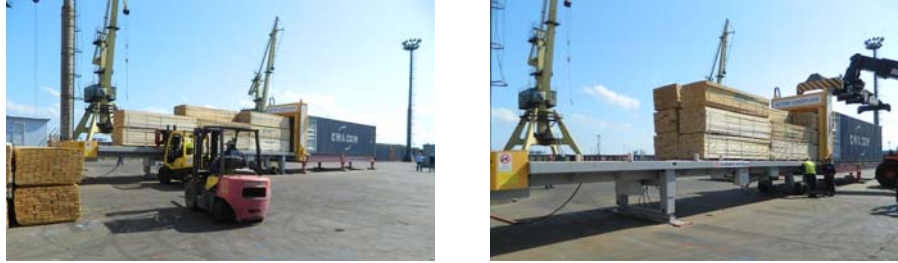
Fig. 6. – The loading stages of the container by means of ALP
