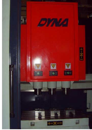
Fig.1 Spindle system of three spindle drilling-tapping vertical machining center
