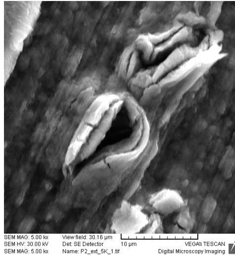
Fig. 10. Cracks in the oxide layer due to thermal stresses(sample P2)
