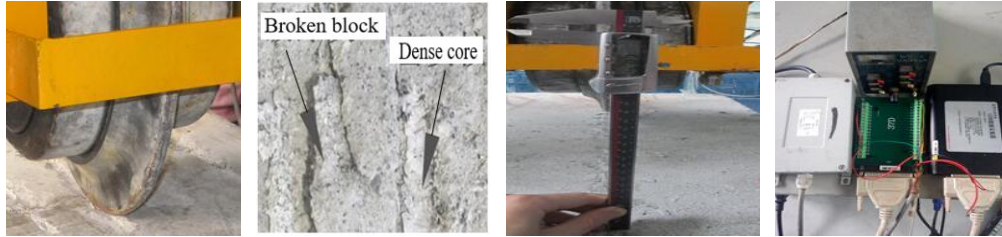
(a) Disc cutter invading rock; (b) Measurement of invasion depth in crater; (c) Measure the depth of invasion; (d) data acquisition Fig. 10 Experimental Process
