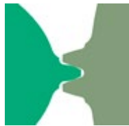
Fig. 5 Geometric model for the plane stress analysis in the case of only one pair of teeth being in contact
