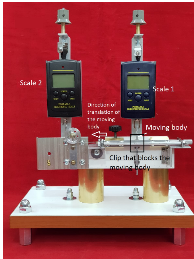
Fig. 2 Apparatus for determining the friction coefficient
