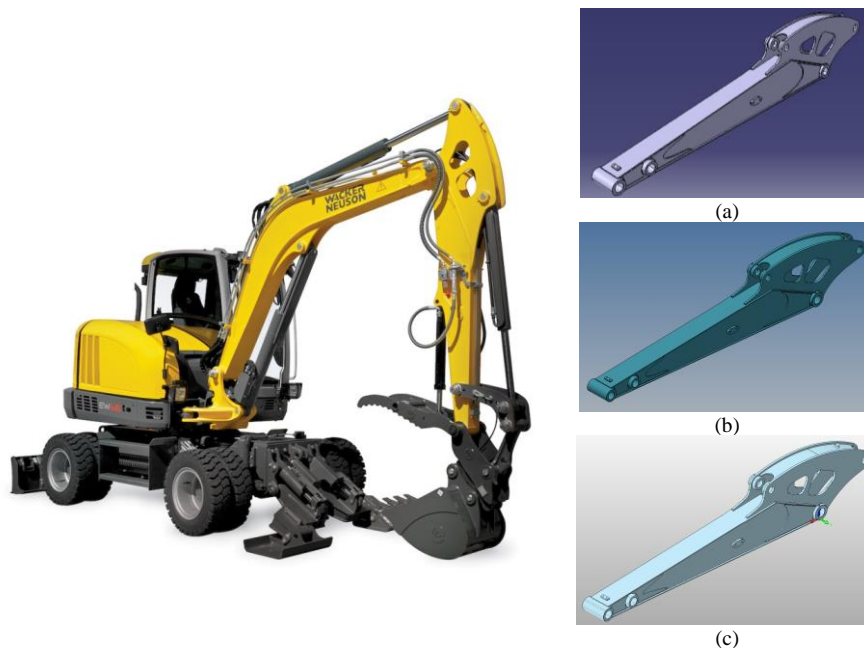
Fig. 6. Excavator Wacker Neuson model EW65 - 3D model of part Loffestiel Lang E14-102: a) CATIA V5R20, b) Autodesk Inventor Professional 2015, c) ZWSOFT ZW3D 2015 SP
