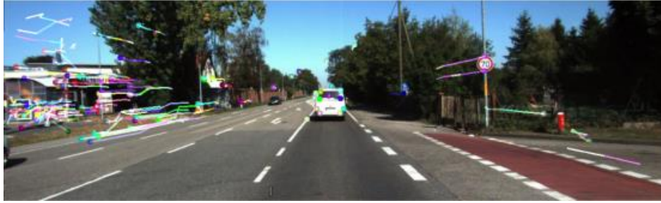
Fig. 3. Sparse optical flow. The dot represents a key point, and the line segment represents a motion trajectory of a key point.
