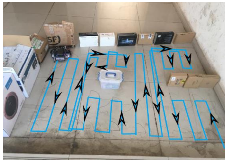
Fig. 18. The route followed by the robot during the comprehensive test.
