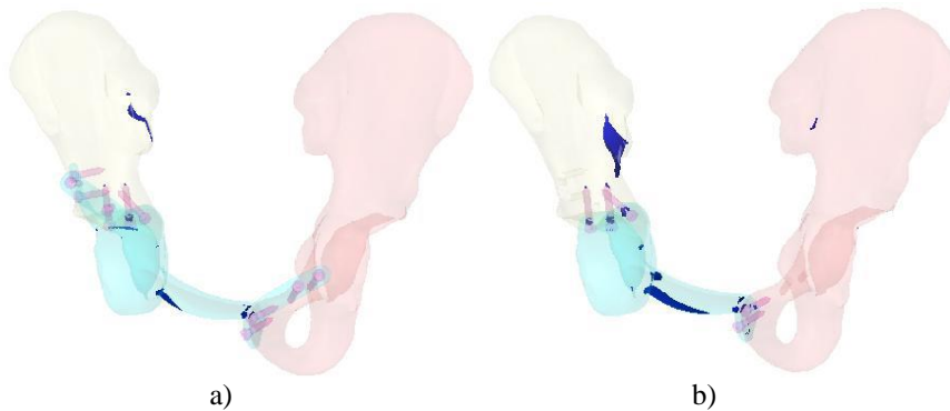
Fig. 8. Design insight diagrams: a) – with additional clamping ears, b) – the simple version
