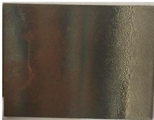
Fig. 4. Specimen No. 2 after deposition of Stellite layer, using metallization process by spray in plasma jet
