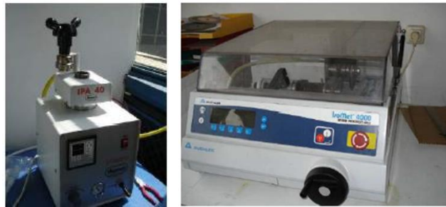
Fig. 5. Die cutting machine for metallographic sample - LAMET-UPB laboratory
