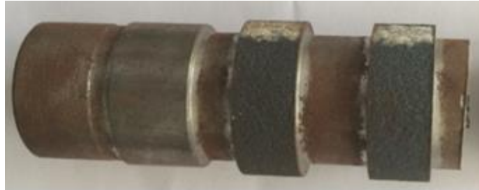
Fig. 3. Specimen No. 1 after deposition of 100 C6 (Rul 1) [4] layer, using electric arc metal spraying
